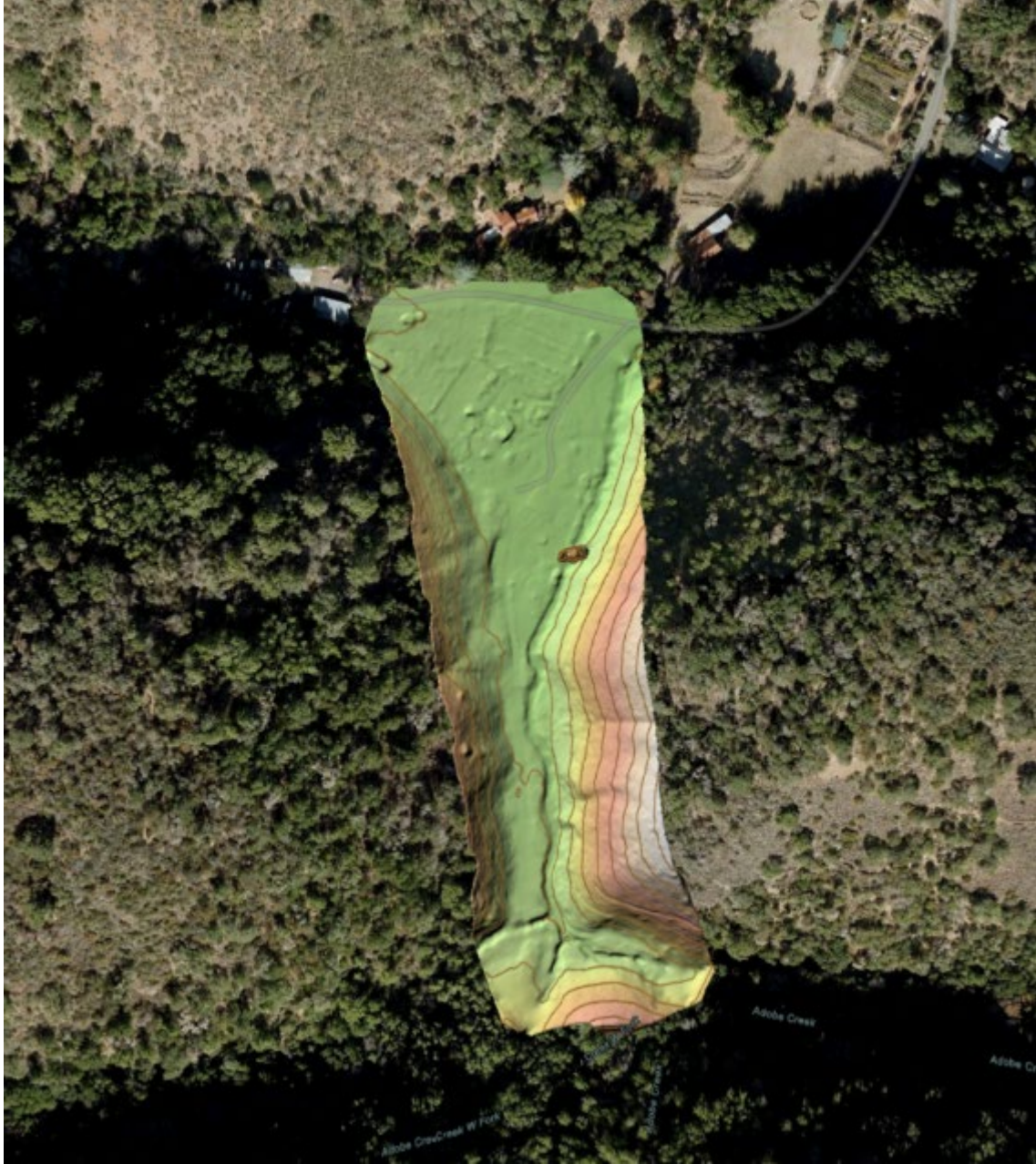
Figure 43. LiDAR Imaging generates high-resolution digital elevation (DEM) maps in spite of forest canopy along Adobe Creek. Prepared by Daniel Cearley from Las Positas College.
