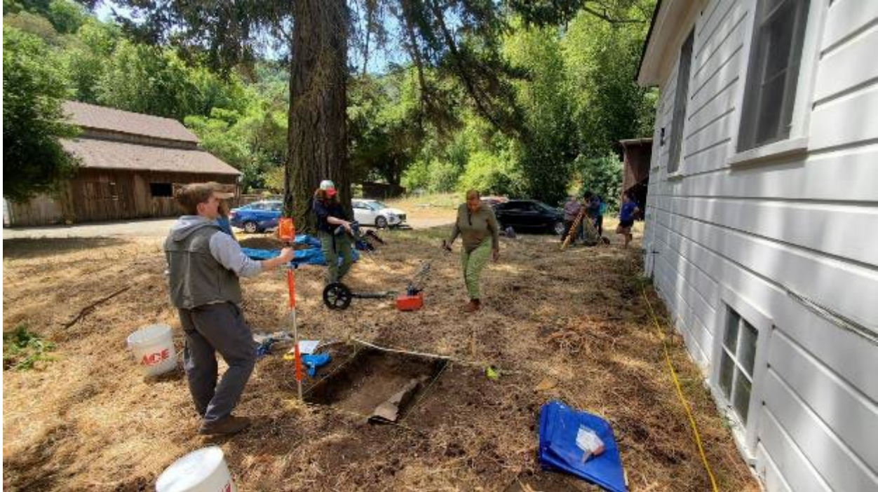
Figure 82. Mapping the location of Unit 4 with the Total Station and simultaneously using the Ground-penetrating radar to scan for more evidence of the pathway and wall – which was not found in the scans (it likely ends or turns toward the house). Total station is located on the site datum. UTM Location of Site Datum is 10S 4133931N 574137E, Elevation 106 meters above sea level.
